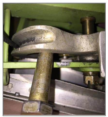
Photo No. 2: Bolt positioned within aileron bell-crank mechanism (The Pilot)
